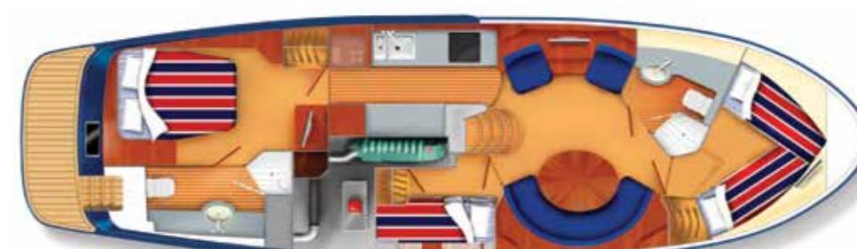
Illustration shows: Owners cabin - double bed, forward cabin - 2 single beds, starboard cabin - 2 bunks
